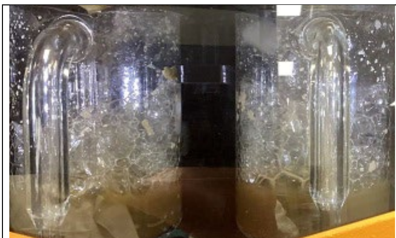
Strong foaming during the boiling with the method "Best Practise" (Sample Soy Drink and Oat Drink)
